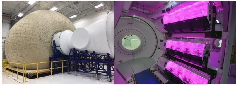
Figure 5. Sierra Space Large Inflatable Fabric Environment (LIFE) mockup. Interior view of habitat showing Astro Garden salad crop production system
