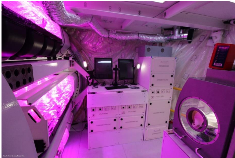
Figure 3. Sierra Space Large Inflatable Fabric Environment (LIFE) mockup. Interior view of habitat showing Astro Garden salad crop production system
