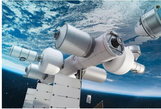
**Figure 5. LIFE modules as part of commercial Orbital Reef Space Station development.**
