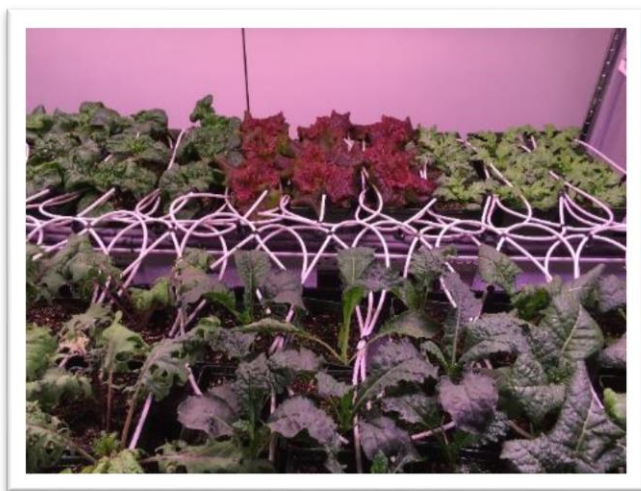
Fig. 3. Left: Test of leafy greens as candidate spaceflight crops. Tests were carried out at 400, 1500, 3000, and 6000 ppm CO 2 to straddle a range of CO 2 levels that might be encountered in space craft like the Intl. Space Station. Right: Heliospectra RX 30 LEDs fixtures used for lighting in the studies.
