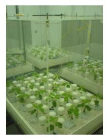
Continuous, Real-Time Measurement of Plant Photosynthesis and Transpiration by Gas Analysis for a Soybean Crop (NJ-NSCORT)
