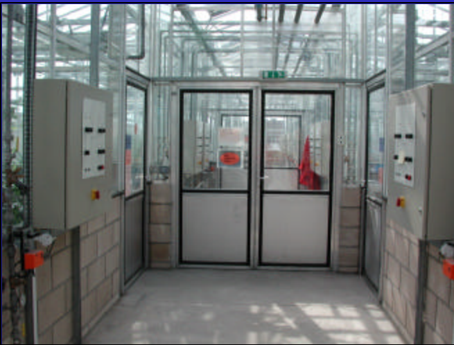
Air lock between high and medium areas
