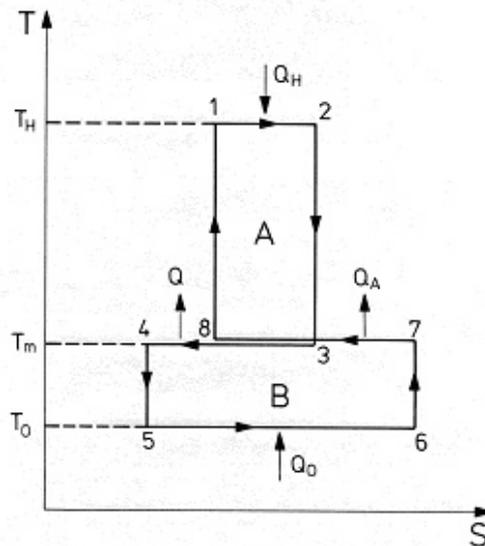
**Figure 3:** Absorption refrigeration cycle
