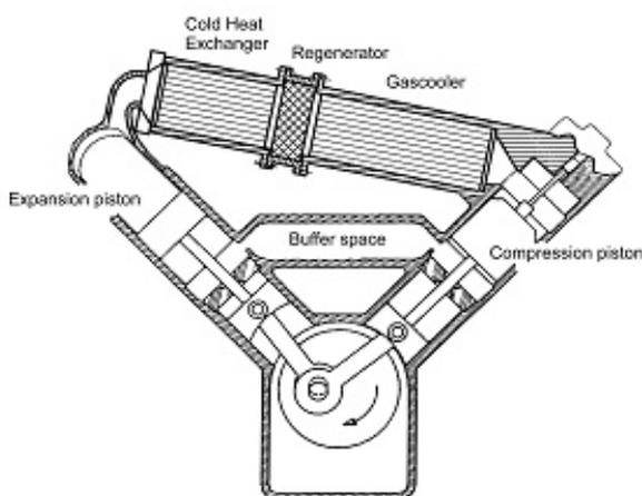
**Figure 8: 161-Stirling refrigerator**
