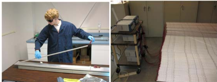
Figure 1. (L) Curing protective coating on LED bar as final step in assembly process. (R) A run of far red LED bars undergoing burn-in testing.
