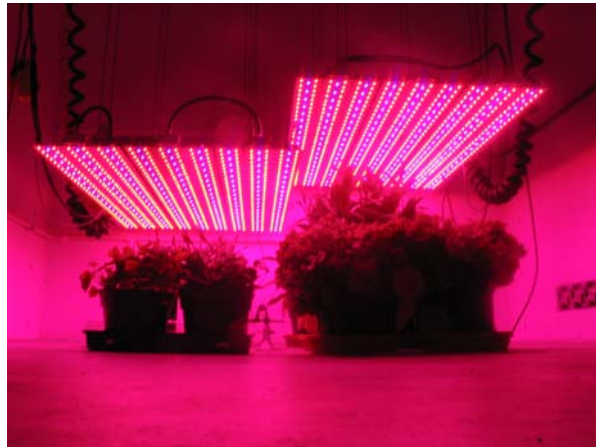
Figure 1. Two ORBITEC built 15 square foot LED arrays.
