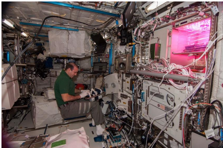
Figure 1. The Veggie Plant Growth in the Columbus Module of the International Space Station. Lighting is provided primarily with red and blue LEDs.
