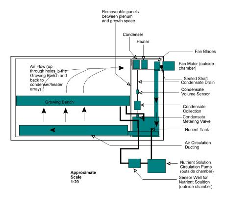
Design schematic of the new hypobaric plant growth chambers to be constructed for the Controlled Environment Research Facility at the University of Guelph
