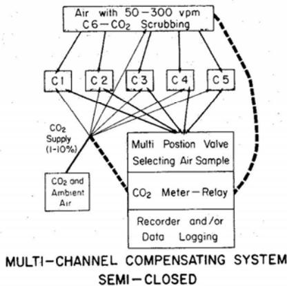
Fig.3.  $CO_2$  control for five growth chambers. A central system which controls the  $CO_2$  concentration of 5 chambers (No. C1 to C5). Air enriched with  $CO_2$  is supplied in amounts proportional to the day time net  $CO_2$  uptake. At night a  $CO_2$  scrubbing chamber (C6) can provide air with low  $CO_2$  content.
