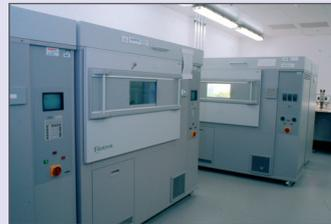
The rooms can all work at either negative or positive pressure dependent on the nature of the exclusion/containment required. All air exchange is through fine filters to prevent organisms being carried out (or in).
