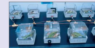
Thrip proof cages are constructed from electrical switchgear boxes.
