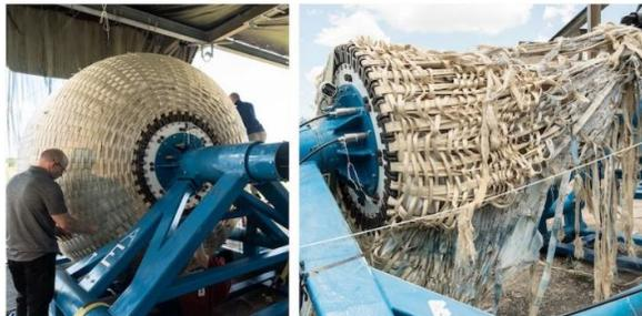
Figure 4. Sierra Space burst testing of 1/3 scale LIFE Habitat prototype. Structure conservatively met structural safety requirements.
