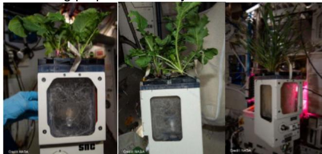
**Figure 1. L>R Radish, Mizuna, and Dwarf Wheat plants grown in aeroponic system on ISS. Water and Nutrient Delivery System with Variable Plant Spacing System**
