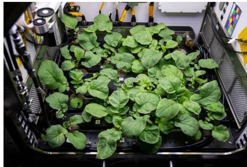
**Figure 3. Radish plants growing inside the Advanced Plant Habitat on ISS (NASA image ss064e013129 Dec. 20, 2020).**
