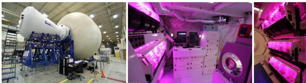
**Figure 4. Sierra Space LIFE module mockup. Left-view of inflatable structure. Center and Right-Interior views of habitat.**
