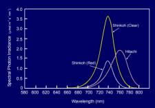
Figure 1. Spectral characteristics of far-red LEDs
