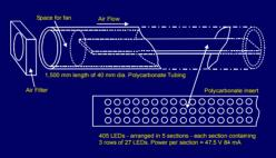
Figure 3. Design of far-red LED arrays
