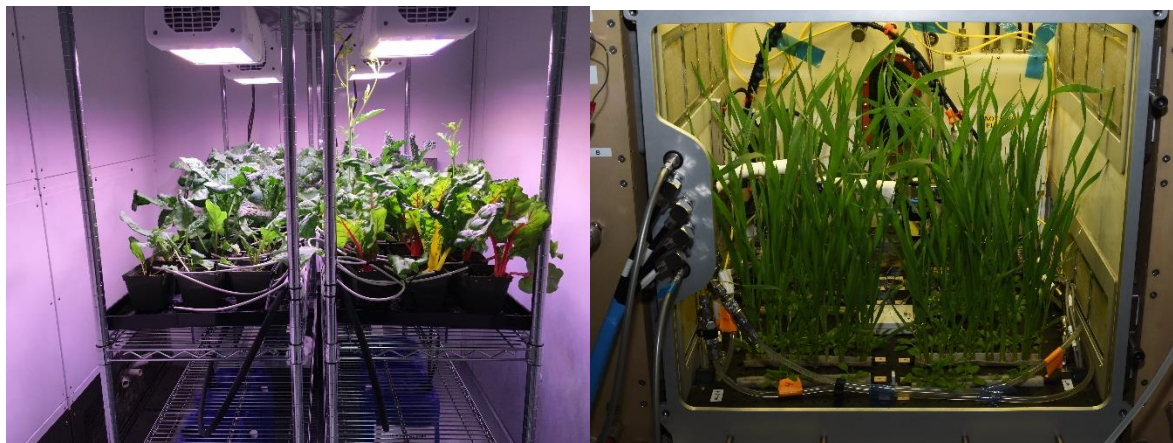
Fig. 2. (Left) Growth chamber testing of “new” salad crops for possible use on the Intl. Space Station. (Right) Ground tests with the Advanced Plant Habitat (APH) recently sent to the Intl. Space Station. The APH has a broad range of environmental control capabilities, with multi-spectral LED lighting, a closed air loop for canopy gas exchange, gravity independent watering system, humidity/condensate recycling, and temp, RH, and CO 2 control.
