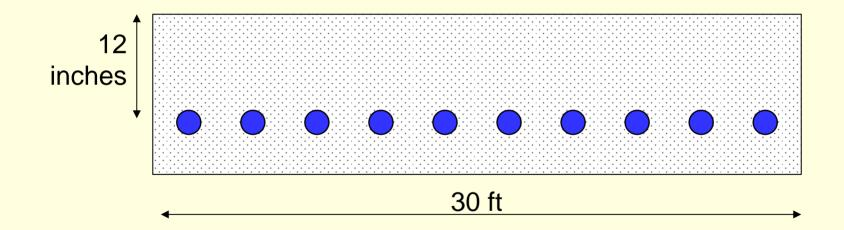
10 HDPE pipes (1.207" outside diameter, 0.079" wall thickness) Depth of pipes below ground level = 12 inches
