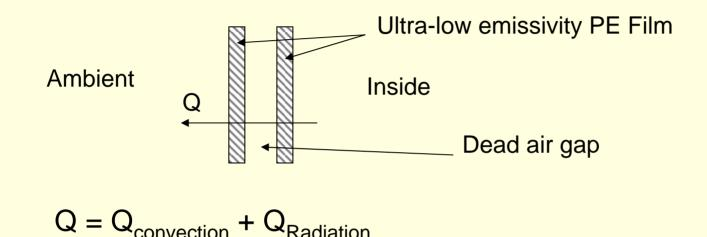
Convection / conduction heat loss is estimated by calculating heat transfer coefficient inside and outside of the tunnel = 6.3 kW
