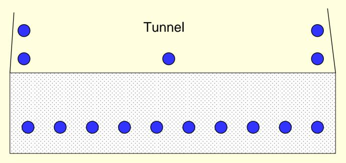
5 additional pipes are used above the ground level Total flow rate of water = 1000 gal/hr Heat in water = 26.85 KW Heat transferred from underground pipes = 7.0 KW Heat transferred from above-ground pipes = 3.5 KW
