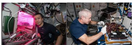
Veggie plant growth unit on the ISS. (L) Veggie flight unit installation, (R) 'Outredgeous' lettuce being harvested from Veggie unit.
