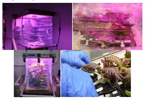
Figure 2. ORBITEC Veggie system. Clockwise from top left; Veggie flight unit, 'Outredgeous' lettuce growing in Veggie unit, lettuce harvest from Veggie plant pillows, Marigold and Zinna in Veggie engineering model.
