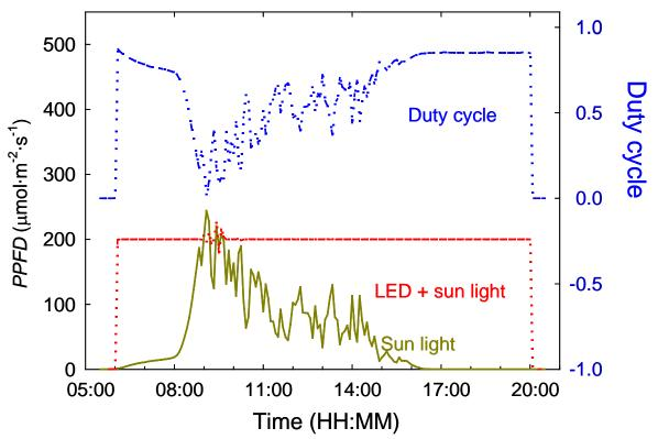
Figure 1. Illustration of the performance of the adaptive LED light. A quantum sensor measures the total amount of light (sun + LED) at the crop level. A microcontroller adjusts the duty cycle of the LED light to provide just enough supplemental light to maintain a stable light level (200  $\mu$ mol·m<sup>-2</sup>·s<sup>-1</sup> in this example) at the top of the canopy. This results in stable light levels for the crop, despite constant changes in the amount of sunlight reaching the crop.
