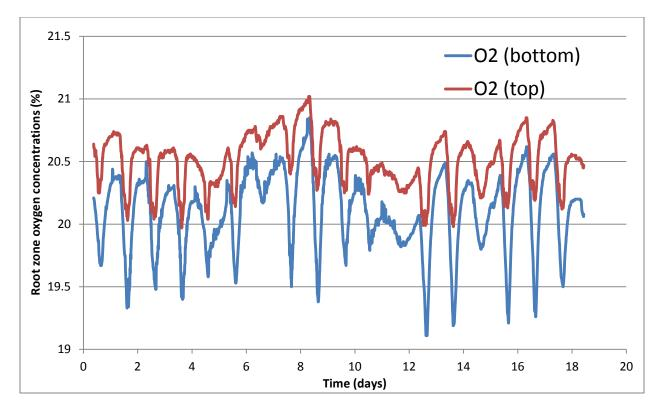
Figure 1. Fluctuations in the oxygen concentration in the root zone of a petunia in a 15-cm pot. One sensor was placed in the top part and one in the bottom part of the pot.
