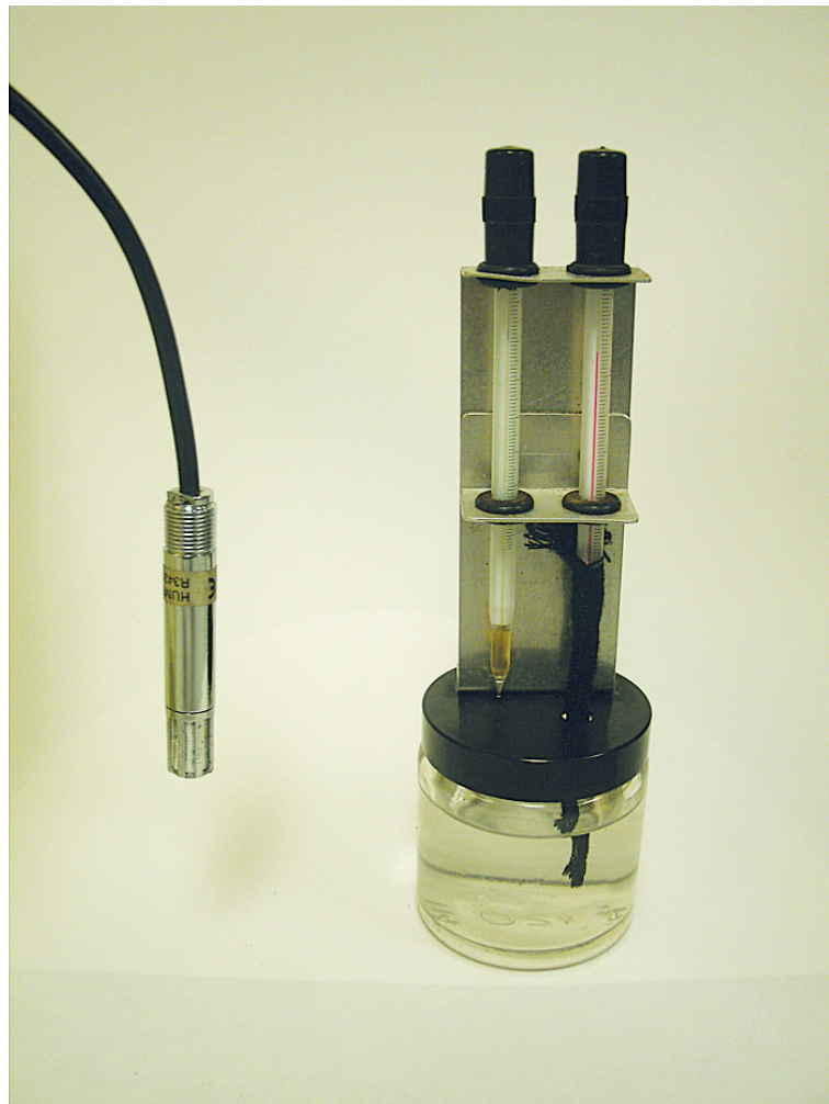
Figure 2. Water vapour (humidity) sensors may be relatively inexpensive capacitance hygrometers (left) or a basic psychrometer (right).
