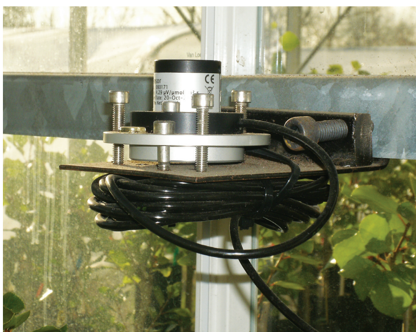
Figure I. A quantum sensor on a levelling platform mounted at the top of the canopy for measuring photosynthetically active radiation (PAR). Radiation sensors should be chosen for the specific purpose required. Positioning should be carefully considered to avoid shading or noise from reflective surfaces. Photograph courtesy of Lancaster Environment Centre, U.K.
