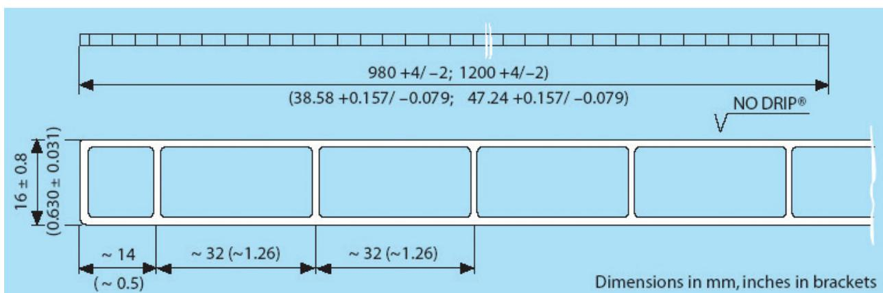
**FIGURE 10. Cross Section of Double Walled Glazing Panel\***
