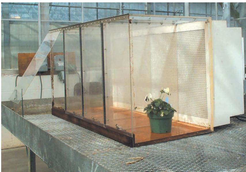
**FIGURE 2.** Negative Pressure Bench-top Containment Unit
