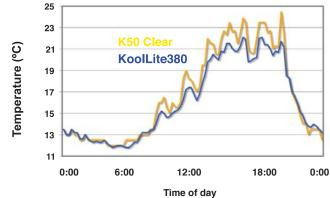
Figure 4. Air temperature (1 m above ground) during August 15, 2007, in high tunnels covered with K50 Clear (yellow), K50 IR/AC (red) and KoolLite380 (blue).
