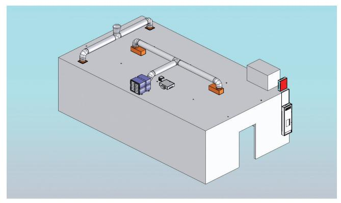
FIGURE 19. Growth Room with HEPA Filtration
