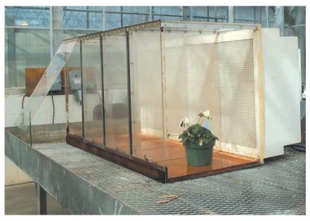
FIGURE 2. Negative Pressure Bench-top Containment Unit
