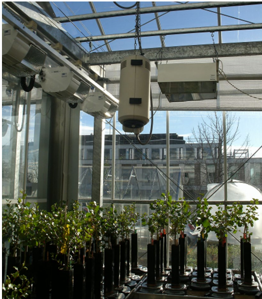
Fig. 3 An aspirated sensor box suspended centrally in free air for recording environmental parameters. The sensors are located inside the box while air is constantly drawn through the box. Sensor (box) type and location along with frequency of sampling and details of data integration should be reported.
